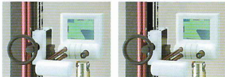
Display of angular grid (1 degree increment) for inspection of Tool cutting edge
