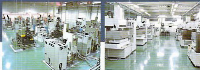
放電加工機群 (左・形彫加工機、右・ワイヤー加工機) Electric-Discharge Machinery Group (Left: Die Sinking Machine, Right: Wire Electric Discharge Machine)
