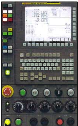
Main operation panel with many rotary switches for intuitive operation.
